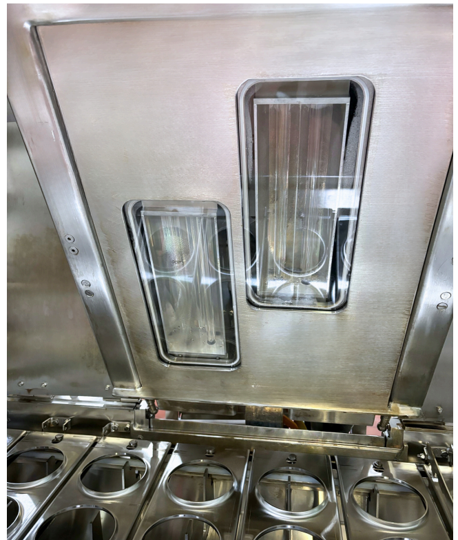
Claranor optical cabinet opened with details on optical cavities
